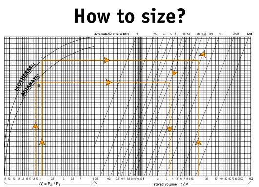
Basic sizing chart for acccumulator used in energy storage.
