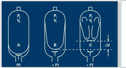
A - Bladder in the precharge position, which means that the accumulator only contains nitrogen. The anti-extrusion system closes the hydraulic orifice which prevents the destruction of the bladder. In low pressure accumulators the bladder rests against the grid. **B** - Position at the minimum operating pressure. There must be a certain amount of fluid between the bladder and the hydraulic orifice, such that the anti-extrusion system does not close the hydraulic orifice.
